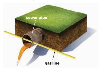
A mechanical rotary device is commonly used to remove a blockage. This process almost always damages the utility line that had been bored through the sewer line. If an electric line is cut, you could be at risk of electrocution. If a gas line is damaged, gas could migrate through the sewer lines into homes and buildings and could result in a major incident/event that may involve death, injury and significant property damage.
