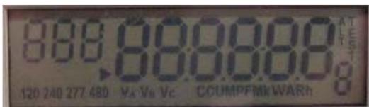
An “all segments” display is shown to verify the LCD segments are all functioning correctly.
