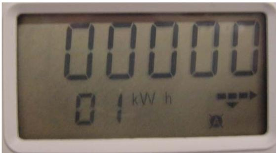
**Display ID 01** represents the total delivered kWh (Energy from Eversource delivered to the customer). This photo also shows a “voltage present” indicator and the LCD segments that indicate the direction and rate of energy flow. Movement from left to right (arrow pointing right) indicates “delivered” kWh. The opposite indicates “received” kWh (excess generation).
