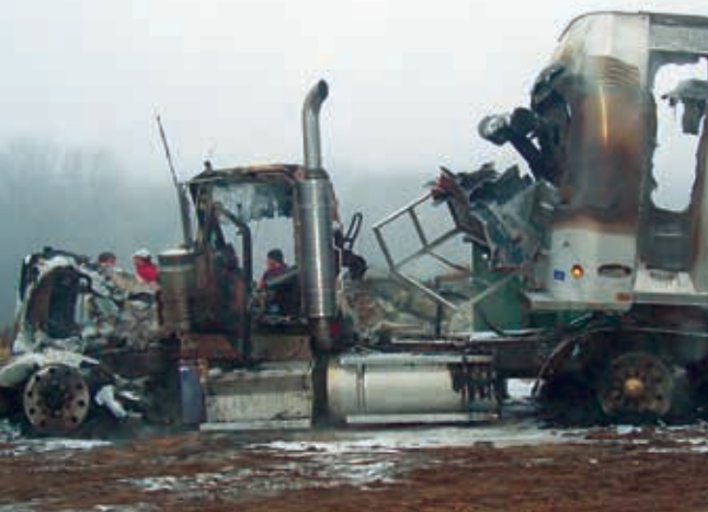
Brooklyn, Conn. — The truck pictured above was being driven with the bed in an elevated position. The bed struck an energized 23,000-volt power line.
