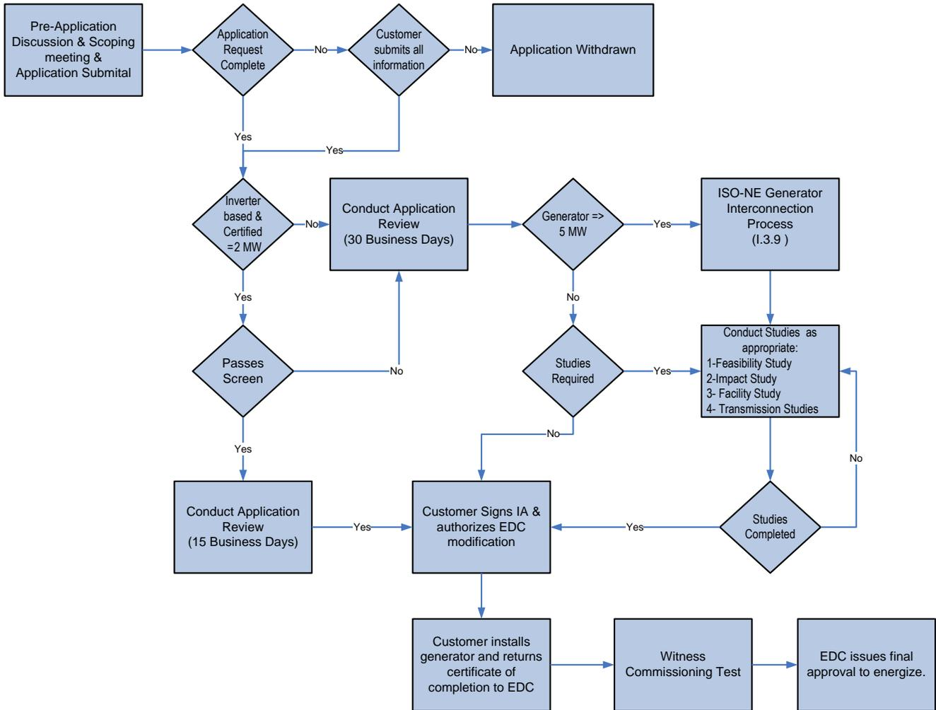
**Additional Process Steps for Generators greater than 5 MW:**
