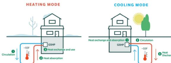
Geothermal systems use wells, piping, and pumps to pull the Earth's heat out of the ground to warm buildings in winter and pumps heat from buildings back into the ground in summer to cool them. This energy, when combined with a ground source heat pump, can be used to comfortably heat and cool indoor spaces year round.
