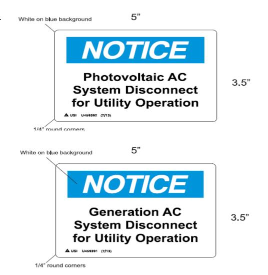
Material Specifications: UV stable materials and adhesive, suitable for outdoor environmental life cycle.
